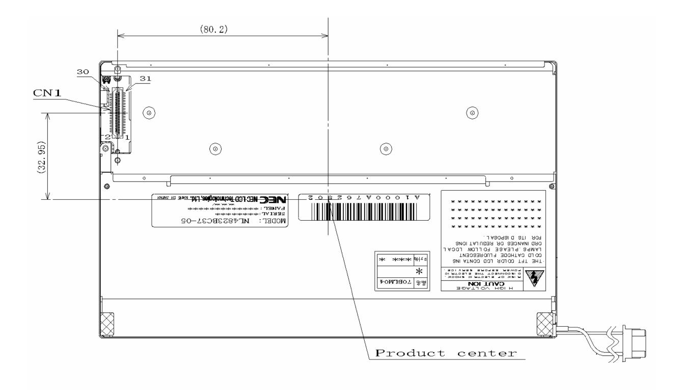
Note1: The values in parentheses are for reference. Note2: The torque for product mounting screws must never exceed 0.147N·m. And the length of mounting screws must be  $\leq$  2.0mm.
