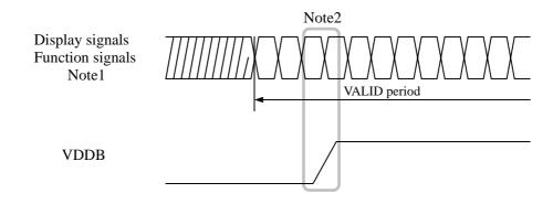
Note1: These are the display and function signals for LCD panel signal processing board. Note2: The backlight should be turned on within the valid period of display and function signals, in
