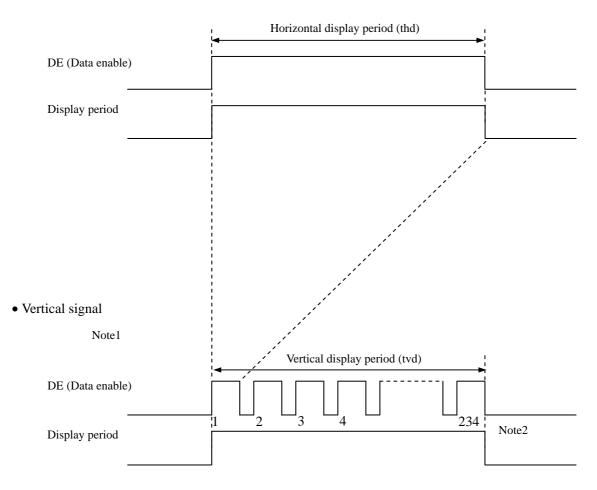
Note1: This diagram indicates virtual signal for set up to timing. Note2: See "**4.9.3 Input signal timing chart**" for numeration of pulse.
