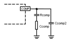
$C_{\text{COMP2}}$  is needed only for high ESR output capacitor Figure 2. Stability Compensation
