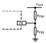
Figure 1. Output Voltage Setting
