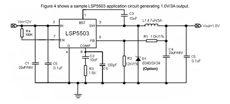
Figure 4. LSP5503 1.0V/3A Output Application
