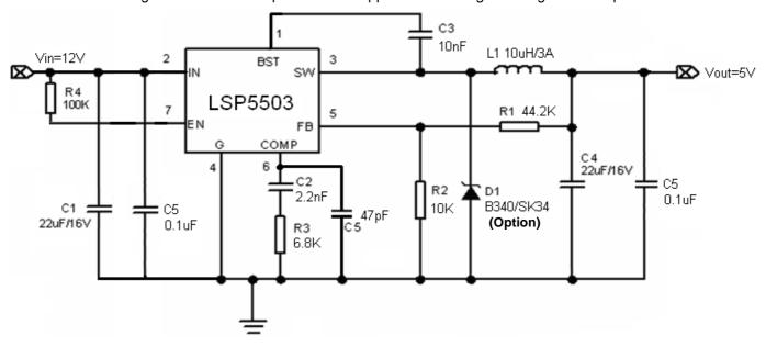
Figure 3. LSP5503 5V/3A Output Application
