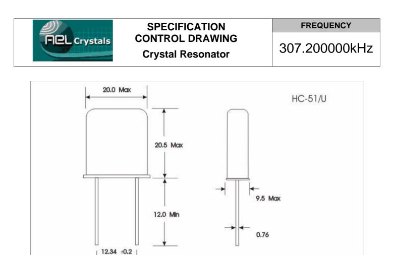
Holder Style Mode Adjustment Tolerance Temperature Stability Operating Temp. Range Load Capacitance Marking HC51U Fundamental ± 50PPM at 25°C ± 100 PPM -10°C to +60°C 30 pF Mark AELX001L\FREQ+WWYY
