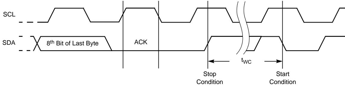
**Nonvolatile Write Cycle Timing**
