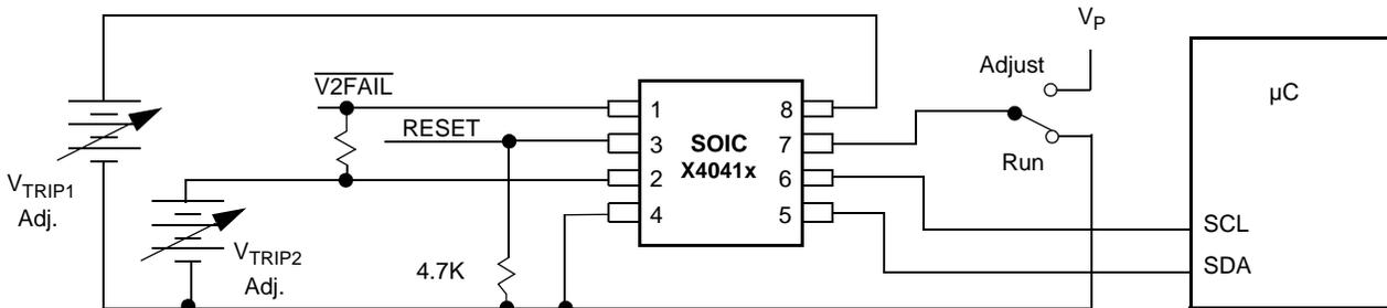
Figure 5.  $V_{TRIPX}$  Set/Reset Sequence (X = 1, 2)
