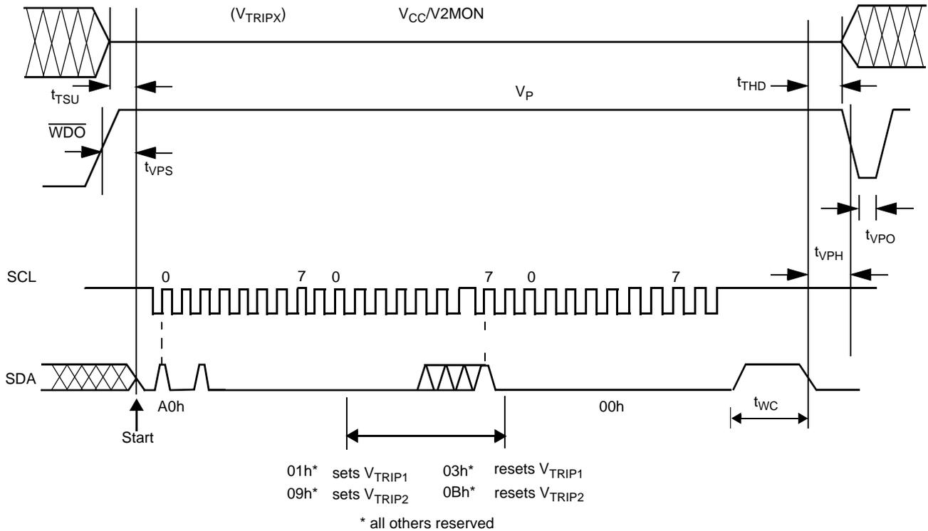
**X40410, X40411, X40414, X40415****V<sub>TRIP1</sub>, V<sub>TRIP2</sub>, Programming Specifications: V<sub>CC</sub> = 2.0–5.5V; Temperature = 25°C**
