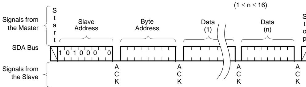
Figure 11. Writing 12 bytes to a 16-byte page starting at location 10.
