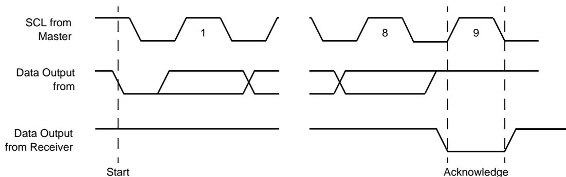
Figure 9. Byte Write Sequence
