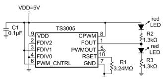
Figure 4: Flashing Railroad Lights with the TS3005
