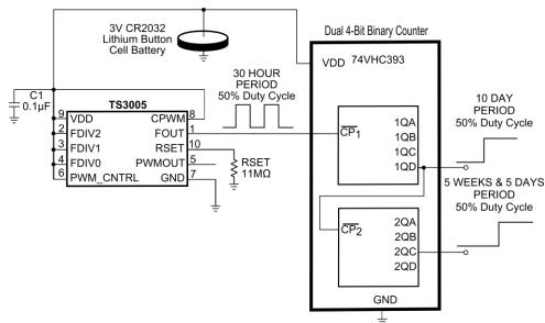
Figure 2: 5 Weeks and 5 Days Counter Circuit
