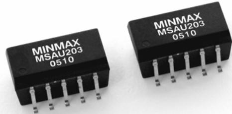
Minmax's MSAU200 1W DC/DC's are in "gull-wing" SMT package, weigh a mere 1.8 grams and meet  $245^{\circ}\text{C}/10\text{sec}$  in solder-reflow for lead free process.
