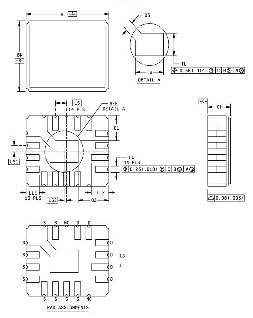
FIGURE 2. Physical dimensions for LCC (2N7261U and 2N7262U).
