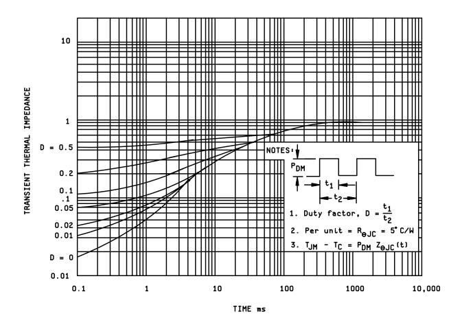
FIGURE 3. Thermal impedance curves.
