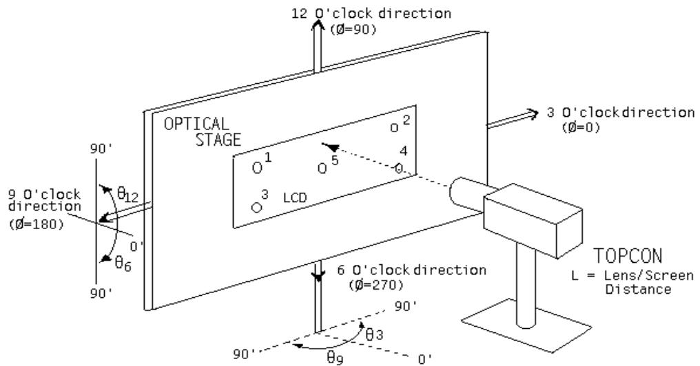
**Figure 2. Average Luminance Measurement & Uniformity Measurement Locations**
