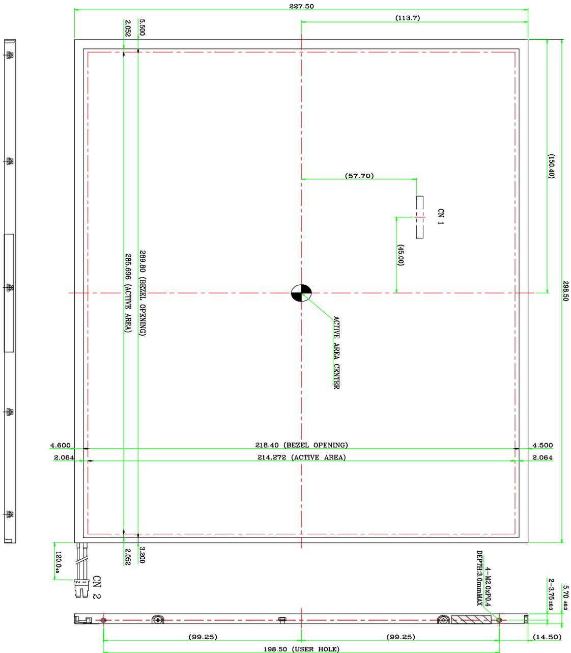
Figure 6. TFT-LCD Module Outline Dimensions (Rear view)
