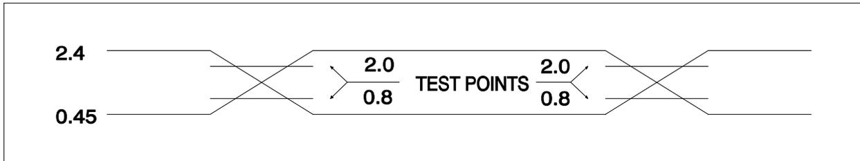
AC Testing: Input are driven at 2.4V for logic "1", and 0.45V for logic "0". Timing measurements are made at 2.0V for logic "1", and 0.8V for logic "0".
