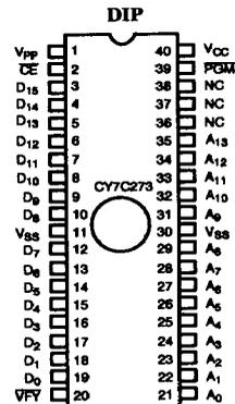
Figure 1. Programming Pinouts
