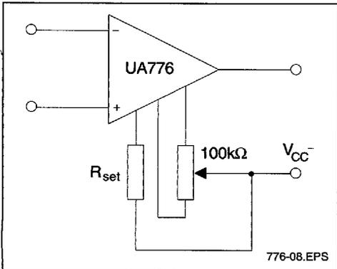
TRANSIENT RESPONSE TIME TEST CIRCUIT
