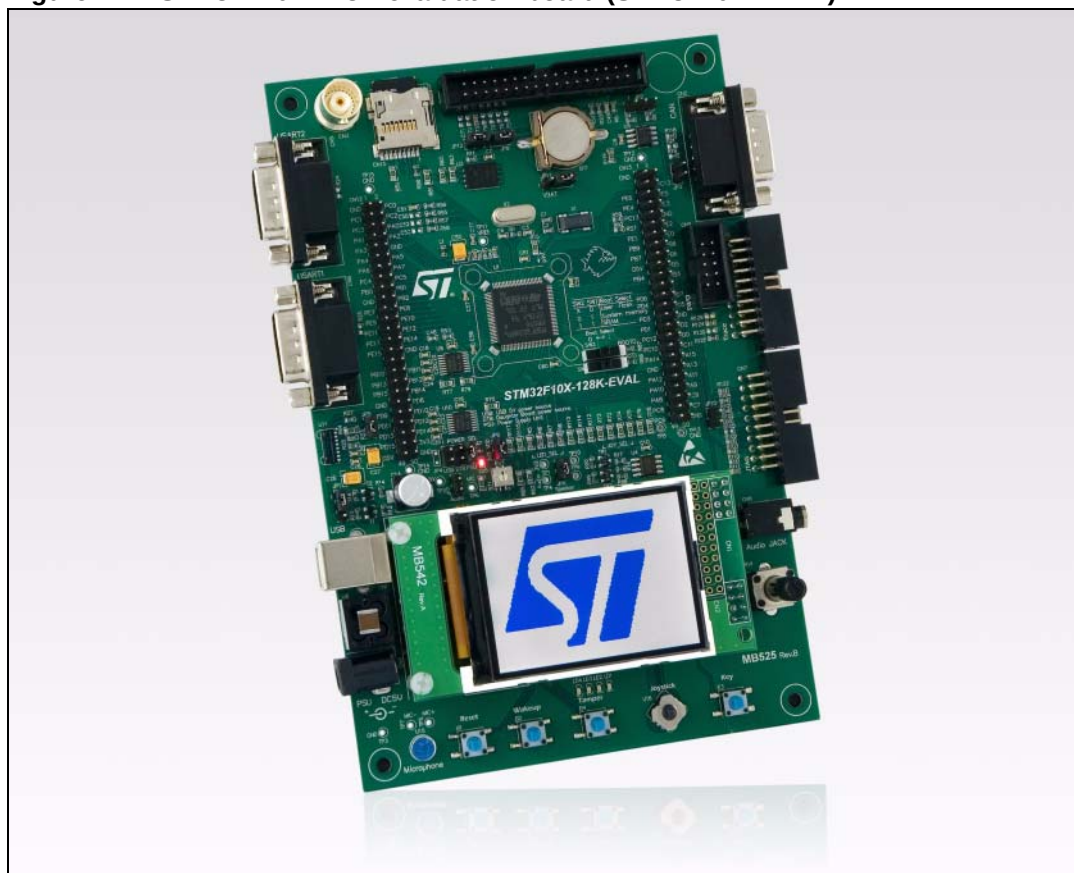
Figure 1. STM32F10X 128K evaluation board (STM3210B-EVAL)
