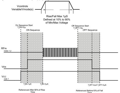
Figure 3: Minimum Recommended ON/OFF Timing Sequence
