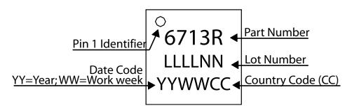
Figure 6: Branding Specification - M45 Package
