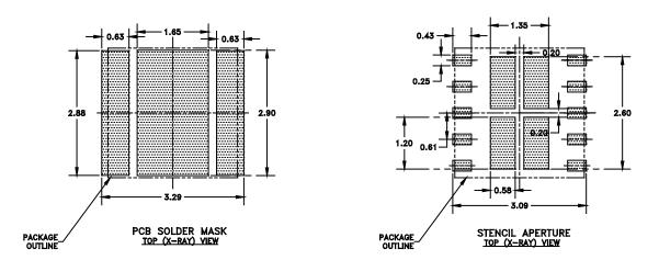
Figure 7: Recommended PCB Layout Information
