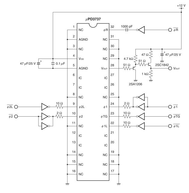
Cautions 1. Leave pins 6, 7, 12, 13, 20, 21, 26, 27 (IC) unconnected.2. Connect the No connection pins (NC) to GND.
