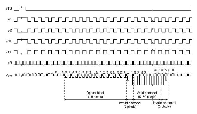
Caution Input the  $\phi$ R pulse continuously during the high level period of  $\phi$ TG.
