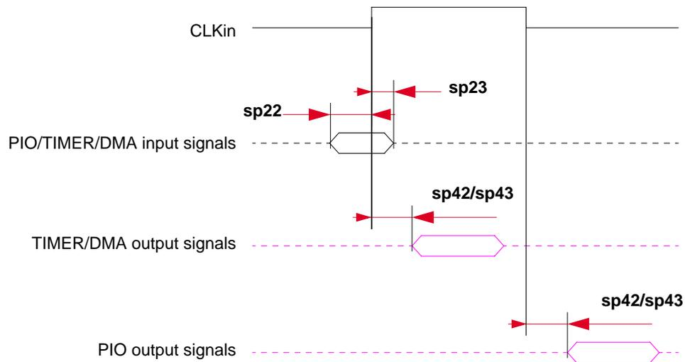
**Figure 6. PIO, Timer, and DMA Signal Diagram**
