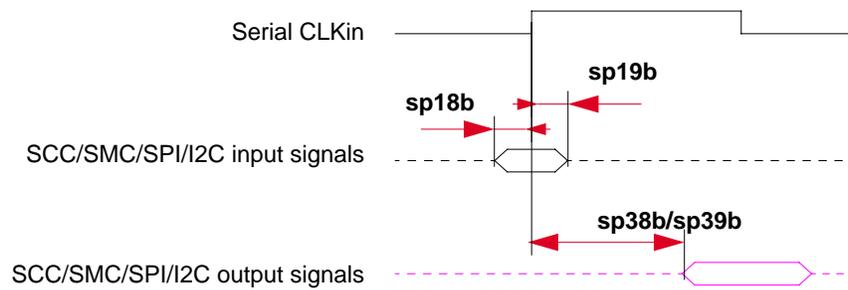
Figure 4. SCC/SMC/SPI/I<sup>2</sup>C External Clock Diagram
