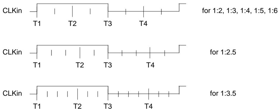
Figure 11. Internal Tick Spacing for Memory Controller Signals
