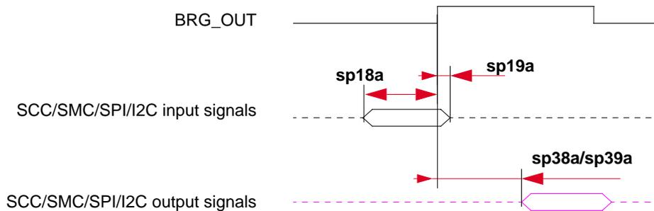
Figure 5. SCC/SMC/SPI/I<sup>2</sup>C Internal Clock Diagram
