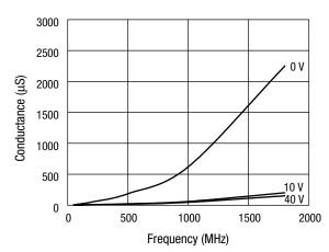
Conductance vs. Frequency and Reverse Voltage
