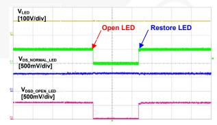
Figure 37. Open LED Protection Operation
