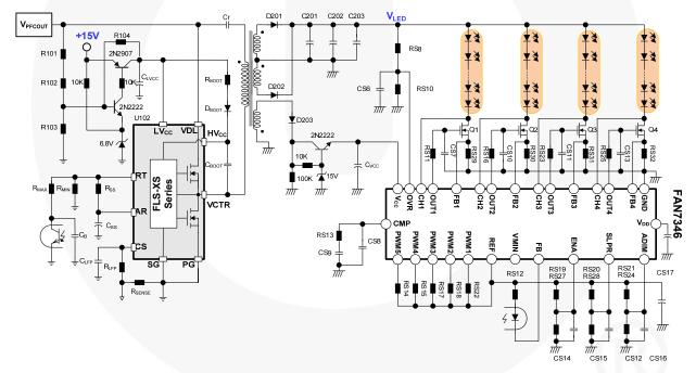
Figure 31. Final Schematic of Half-Bridge LLC Resonant Converter for Multi Channel
