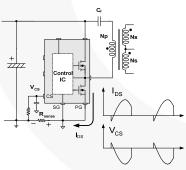
Figure 26. Half-Wave Sensing
