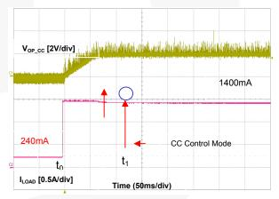
Figure 36. Constant-Current Control Waveforms
