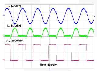
Figure 32. Operation Waveforms at Full-Load Condition
