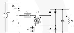
Figure 1. Half-Bridge, LC Series Resonant Converter
