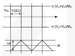
Figure 20. Flux Density Swing
