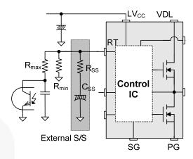
Figure 24. Typical Circuit Configuration for RT Pin
