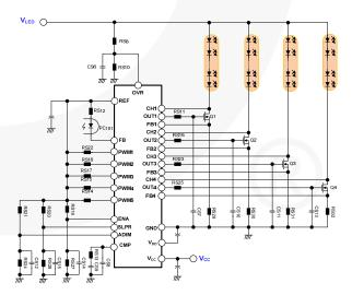
Figure 29. Example of CC and OVR Feedback Circuit
