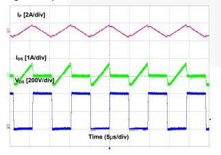
Figure 33. Operation Waveforms at No-Load Condition
