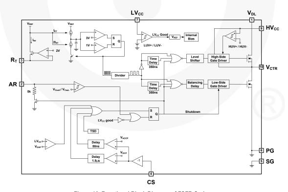
Figure 16. Functional Block Diagram of FSFR-Series
