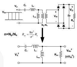
Figure 6. AC Equivalent Circuit for LLC Resonant Converter
