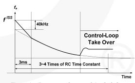
Figure 25. Frequency Sweep of the Soft-Start
