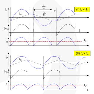
Figure 11. Waveforms of Each Operation Mode
