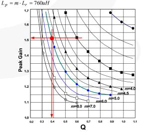
Figure 19. Resonant Network Design Using the Peak Gain (Attainable Maximum Gain)
