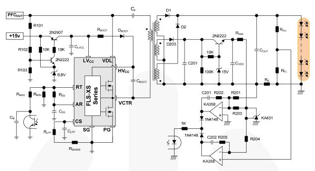
Figure 17. Reference Circuit for Design Example of LLC Resonant Half-Bridge Converter
