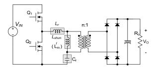
Figure 2. Half-Bridge LLC Resonant Converter
