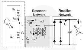
Figure 3. Schematic of Half-Bridge LLC Resonant Converter
