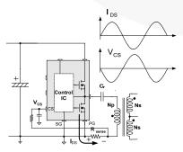
Figure 27. Full-Wave Sensing
