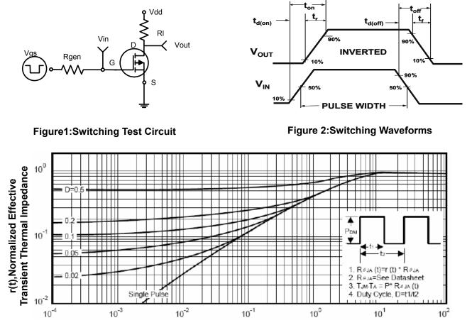
Square Wave Pluse Duration(sec) Figure 3: Normalized Maximum Transient Thermal Impedan
