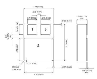
Bipolar NPN Device in a Hermetically sealed
