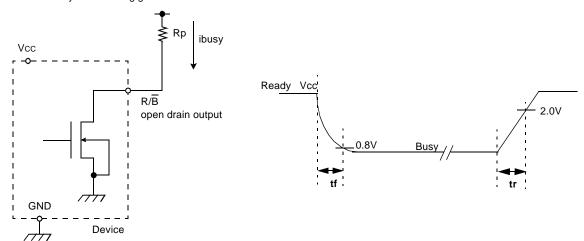
Figure 16 Rp vs tr ,tf & Rp vs ibusy
