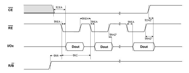
NOTES: Transition is measured ±200mV from steady state voltage with load. This parameter is sampled and not 100% tested.
