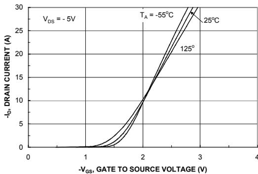
Figure 5. Transfer Characteristics.
