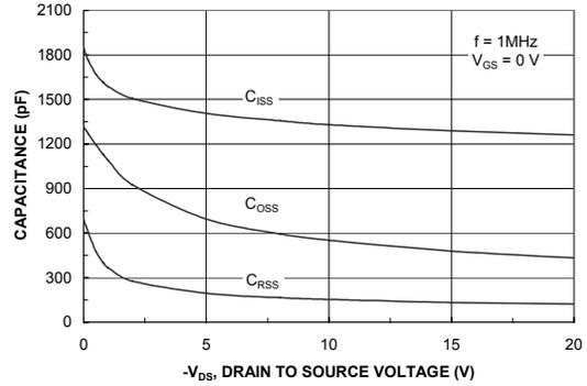
Figure 8. Capacitance Characteristics.
