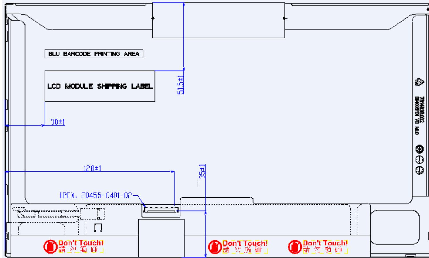
Note: Prevention IC damage, IC positions not allowed any overlap over these areas.
