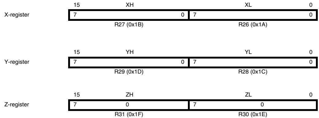
Figure 5. The X-, Y-, and Z-registers
