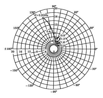
$\begin{array}{l} S_{12e} \\ V_{CE} = 10V \\ I_{C} = 20 \text{mA} \\ Ta = 25 ^{\circ}C \end{array}$
