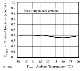
Figure 6. Sensitivity vs. Ambient Temperature
