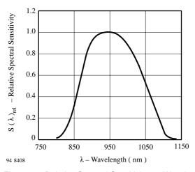
Figure 11. Relative Spectral Sensitivity vs. Wavelength
