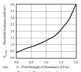
Figure 4. Threshold Irradiance vs. Field Strength of Disturbance
