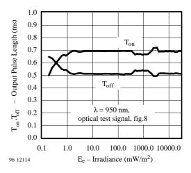
Figure 10. Output Pulse Diagram
