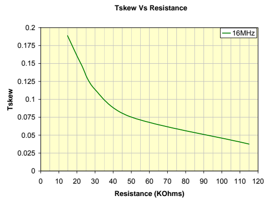
Fig12: Tskew Vs Resistance (16MHz, FS=1)
