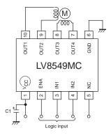
\* Bypass capacitor (C1) connected between  $V_{CC}$ -GND of all examples of applied circuit recommends the electric field capacitor of  $0.1\mu A$  to  $10\mu A$ .
