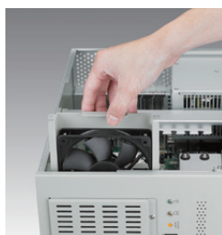
Easy-to-maintain cooling fan
