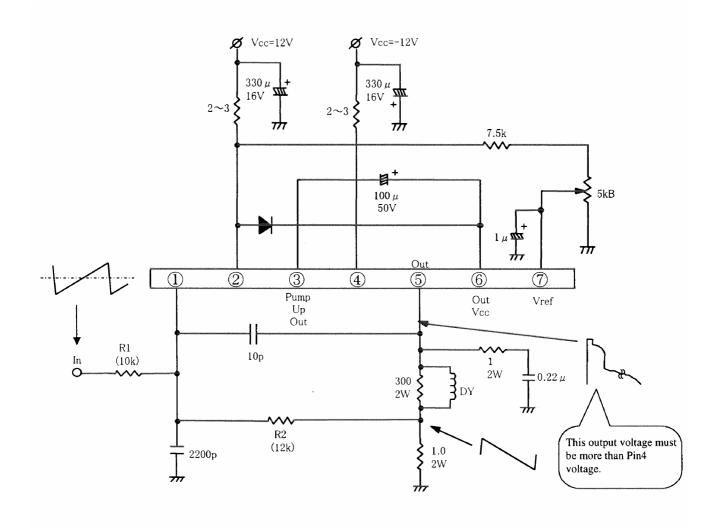
In order to get required gain, it is necessary to adjust the R1 and R2.
