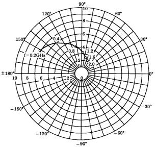
$\begin{array}{c} S_{12e} \\ V_{CE} = 6V \\ I_{C} = 7mA \\ Ta = 25^{\circ}C \end{array}$
