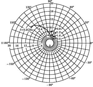
$S_{12e}$   $V_{CE} = 6V$   $I_{C} = 3mA$   $T_{a} = 25^{\circ}C$
