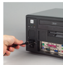
Plug ring-lock securely fastens the power cord
