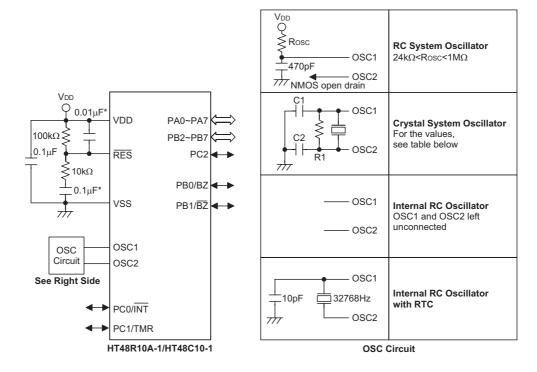
Note: The resistance and capacitance for reset circuit should be designed to ensure that the VDD is stable and remains in a valid range of the operating voltage before bringing RES to high.
