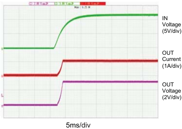
Short Circuit Protection
