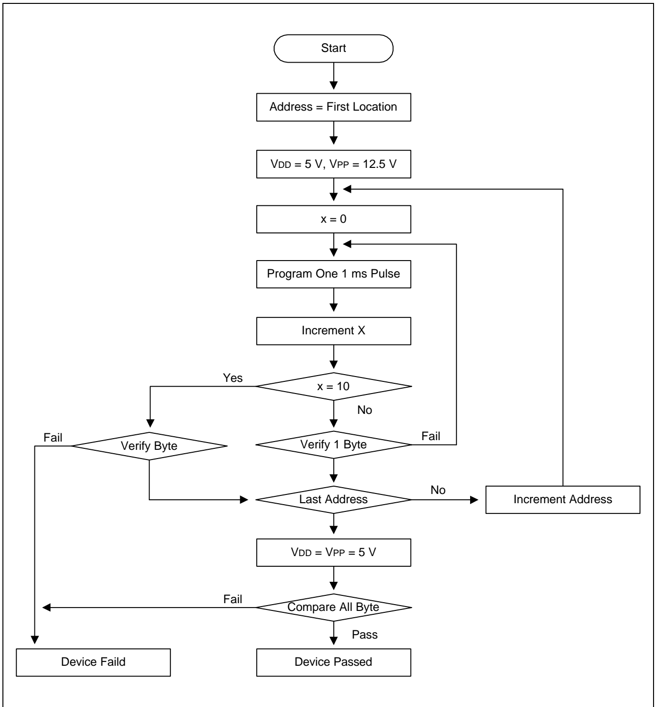
Figure 17-2. OTP Programming Algorithm
