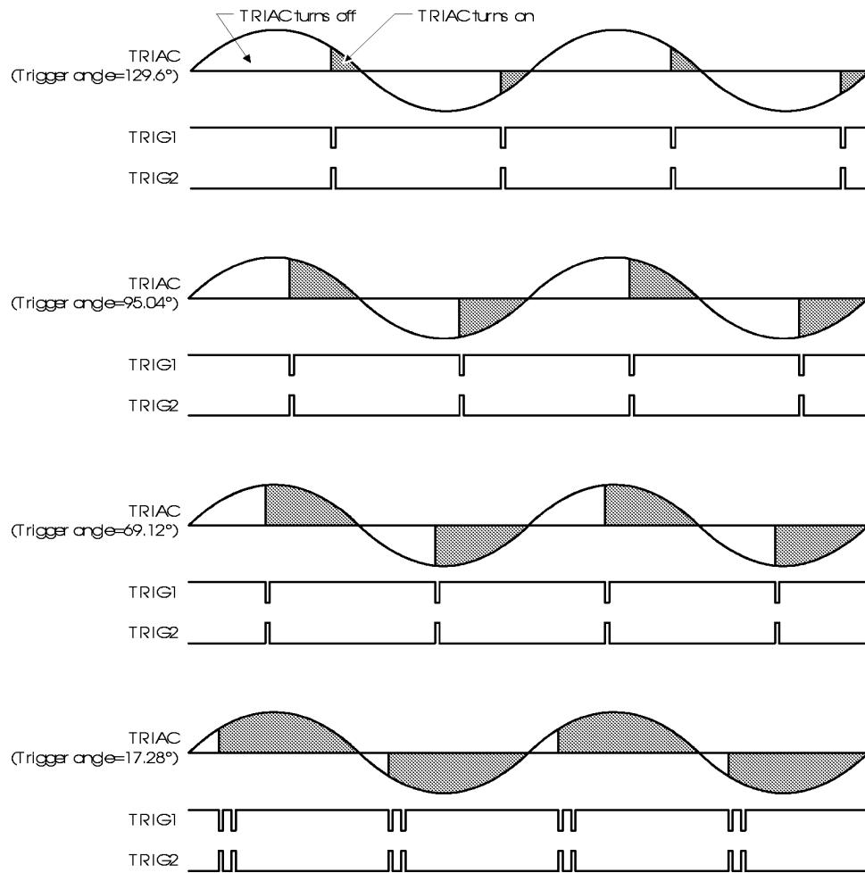
**On/off trigger angle (Fosc=400KHz)**
