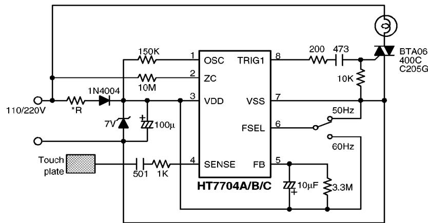
\* Note: 1)  $R=22\text{K}\Omega/2\text{W}$  when the AC power supply is 110V.
