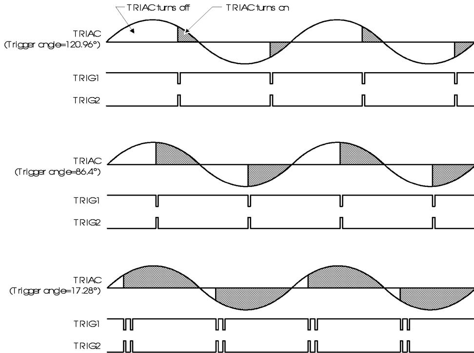
4 steps trigger angle (Fosc=400KHz)
