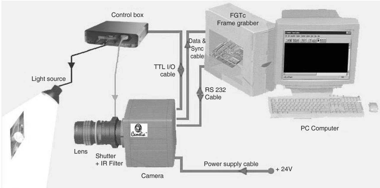
Figure 2. CameraLink Camera Imaging System
