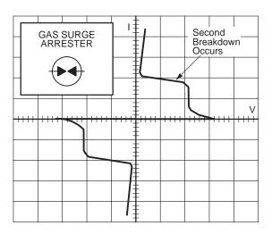
In this plot, it is possible to observe that the GDT's response is relatively slow, and sometimes this factor could be very critical for telecom applications in which the fast response is needed. In addition, as a result of this slow response, some gas tubes' electrodes burn out after a few hundred hits.
