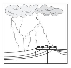
Lightning causes a large shift in ground potential near a lightning strike. These shifts can reach as high as 50 KV. Large magnetic fields from lightning strikes may also cause problems.
