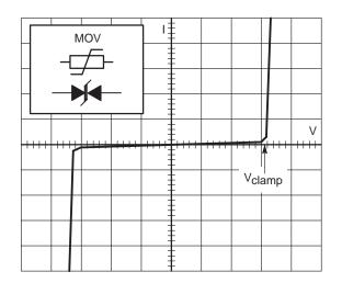
When a MOV reaches its Zener voltage, it starts to dissipate power, so this is why, if a high transient voltage occurs, the MOV may be damaged because of the high power dissipation that this transient may cause. At the same time, it is very common that the MOV becomes degraded each time it is activated.
