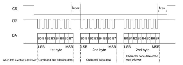
\* When data is written to RAM (DCRAM, ADRAM, CGRAM) continuously, addresses are internally incremented automatically.
