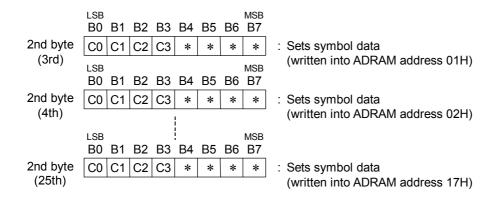
The symbol data setting up to 24 digits is completed. To set symbol data from ADRAM address 00H continuously. Specify a dummy symbol data between ADRAM addresses 18H and 1FH. (To increment the ADRAM address automatically and set it to 00H)
