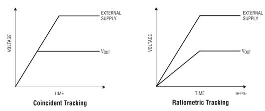
Figure 5(a). Two Different Modes of Output Tracking
