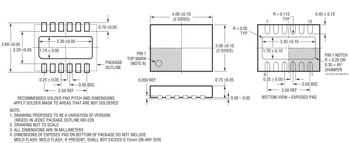
DE/UE Package 12-Lead Plastic DFN (4mm  $\times$  3mm)
