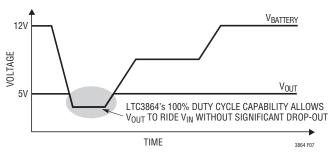
Figure 7. Typical Automotive Cold Crank
