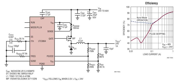
24V to 60V Input, 24V/1A Output at 750kHz
