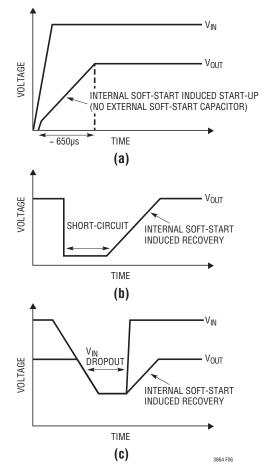
Figure 6. Internal Soft-Start (a) Allows Soft Start-Up without an External Soft-Start Capacitor and Allows Soft Recovery from (b) a Short-Circuit or (c) a  $V_{\rm IN}$  Dropout
