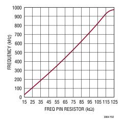
Figure 2. Switching Frequency vs Resistor on FREQ
