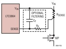
Figure 3. Inductor Current Sensing
