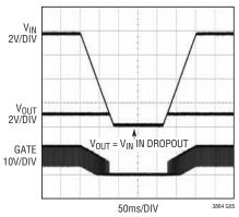
$\begin{array}{l} V_{IN} \mbox{ TRANSIENT: 12V TO 4V} \\ \mbox{ AND BACK TO 12V} \\ V_{OUT} = 5V, \mbox{ I}_{LOAD} = 100 \mbox{mA}, \mbox{ FIGURE 8 CIRCUIT} \end{array}$
