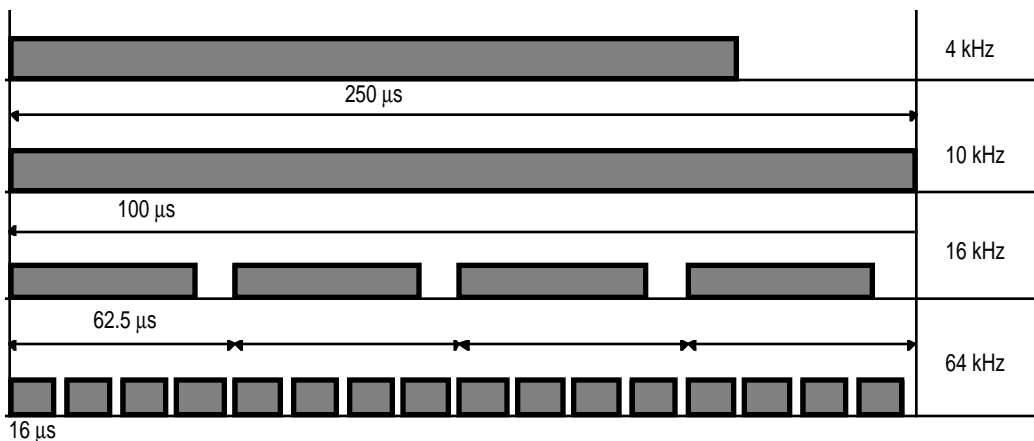
Figure 38. PWM Waveform of the Active Region (for a 6-bit PWM data)
