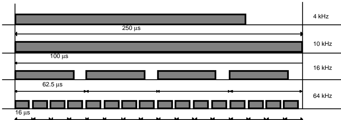
Figure 37. PWM Waveform (shaded area shows the active region)
