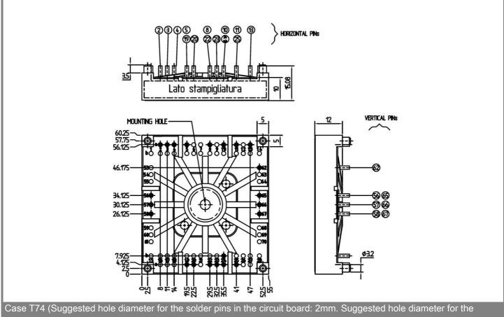
mounting pins in the circuit board: 3,6mm )
