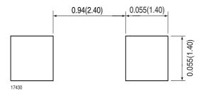
Layout for  $R_{\theta JA}$ Thickness: Fiberglass 0.0059 in. (1.5 mm)
