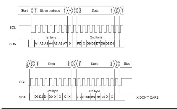
The standard data transfer to this device consists of four bytes : the slave address of the first byte and the data of the second, third and four bytes.
