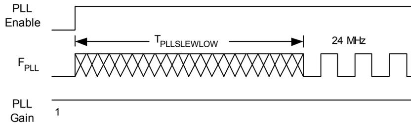
**Figure 8. External Crystal Oscillator Startup Timing Diagram**
