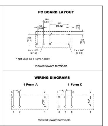
Dimensions in inches with metric equivalents in parentheses. Tolerance: ± .010"
