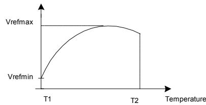
2. The temperature coefficient is defined as the slopes (positive and negative) of the voltage vs temperature limits whithin which the reference voltage is guaranteed.
