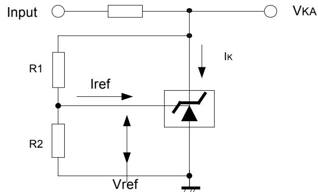
Figure 3: Test Circuit for  $I_{off}$
