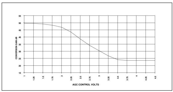
Fig.4 Typical AGC characteristic
