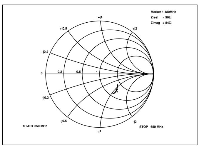
Fig.3 Typical RF input impedance
