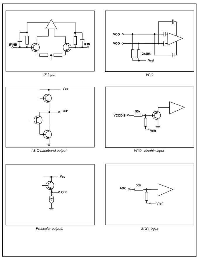
Fig. 6 I/O port peripheral circuitry
