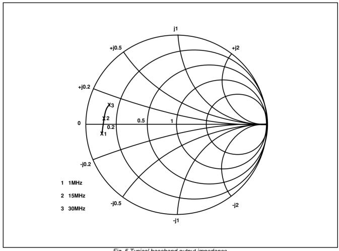
Fig. 5 Typical baseband output impedance
