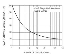
FIG.4 MAXIMUM NON-REPETITIVE FORWARD SURGE CURRENT
