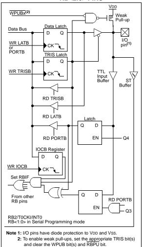
FIGURE 9-3: BLOCK DIAGRAM OF RB3 PIN
