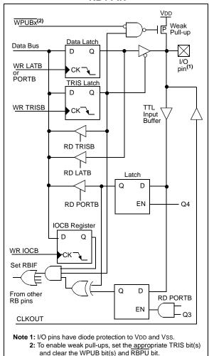
FIGURE 9-5: **BLOCK DIAGRAM OF RB5 PIN**
