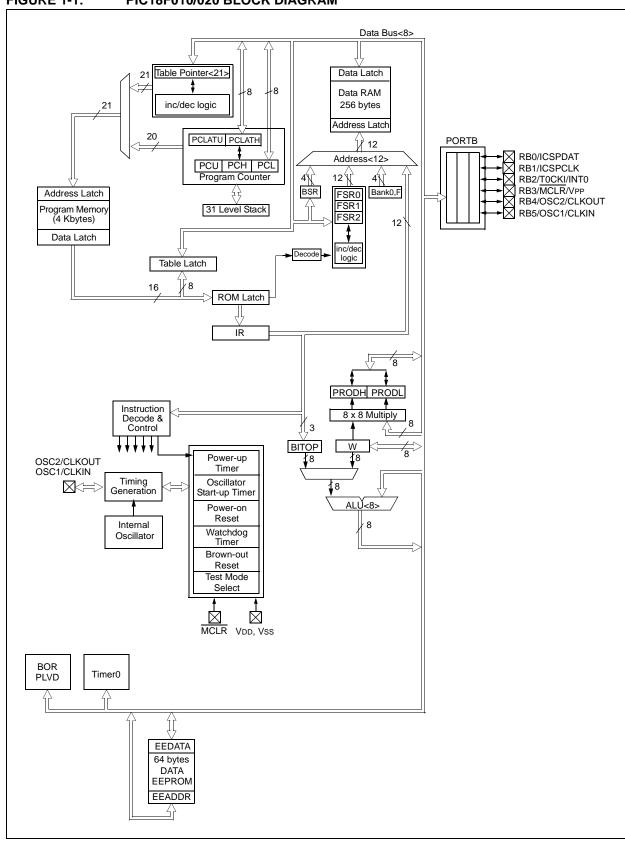
FIGURE 1-1: PIC18F010/020 BLOCK DIAGRAM
