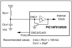
In the RC mode, the oscillator frequency divided by 4 is available on the OSC2 pin. This signal may be used for test purposes, or to synchronize other logic. In the RCIO mode, the OSC2 pin becomes a general purpose I/O pin. This pin is RB4 of PORTB.
