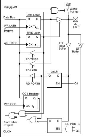
Note 1: I/O pins have diode protection to VDD and Vss.
