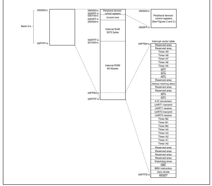
Fig. 1 Memory map of M37906F8CFP, M37906F8CSP (Single-chip mode)
