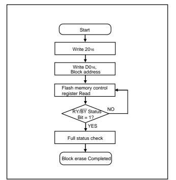
Fig. 10 Block erase flowchart
