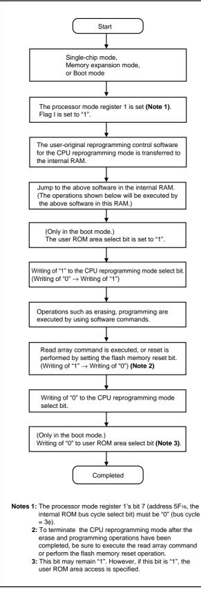
Fig. 8 CPU reprogramming mode set/termination flowchart
