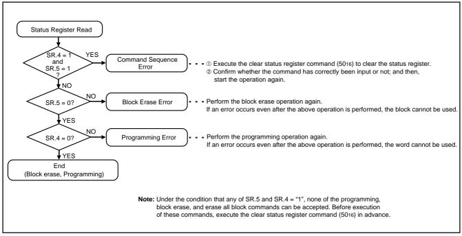
Fig. 11 Full status check flowchart and actions to be taken if an error has ocurred
